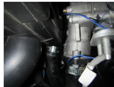
Figure 5: The inlet and outlet water temperature sensors of radiator on the vehicle
